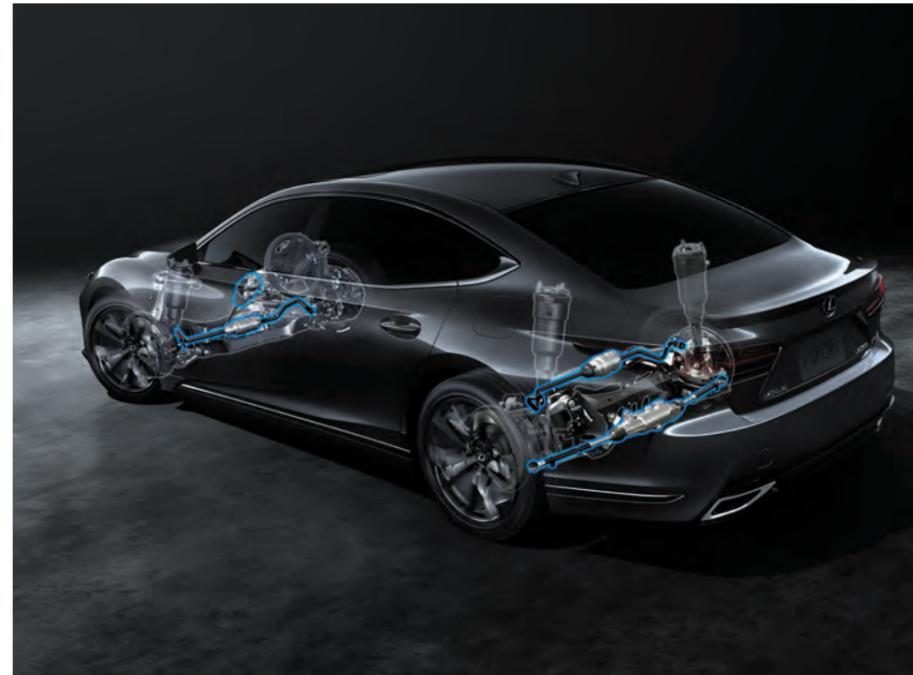
VDIM (With integrated active steering control) + LDH
