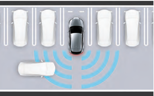
PKSB (Parking Support Brake) While the vehicle is travelling at a low speed, if there is a possibility of contact with a static object around the vehicle, a vehicle or a pedestrian approaching from the rear, the system applies drive force control and brake control. Detection covers a wide area surrounding the vehicle, helping to avoid minor collisions and reduce damage.
