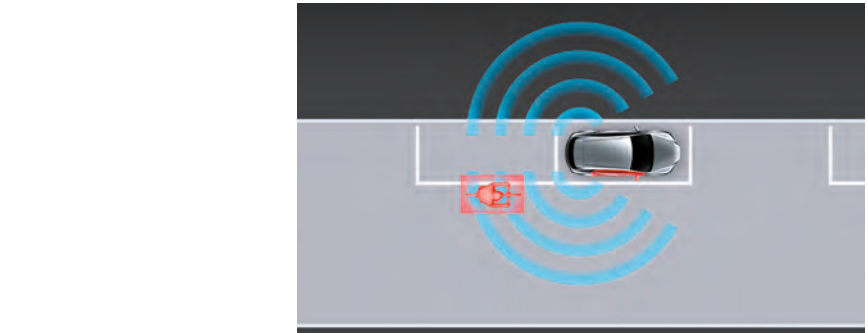
BSM (Blind Spot Monitor) During lane changes, the BSM uses rear lateral side millimeter-wave radar to detect vehicles present in the blind spots (areas in adjacent lanes that cannot be seen using the outer mirrors), and alerts the driver using an indicator in the outer mirror and a buzzer.
